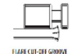
*Tube cutter with the grooves in the roller clearly visible and use.*
