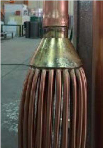
Each section of the cooling coil is supplied separately with refrigerant. Instead of using a separate TEV for each section of the cooling coil, a single TEV with a liquid distributor is used. See figure 8. This distributor is attached directly to the TEV.
